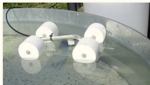
TS 265 sensor with float for evaporation tank
