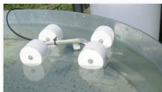
TS 265 sensor with float for evaporation tank
