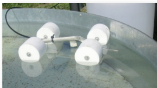
TS 265 sensor with float for evaporation tank
