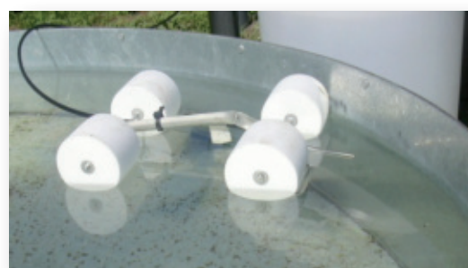
TS 265 sensor with float for evaporation tank
