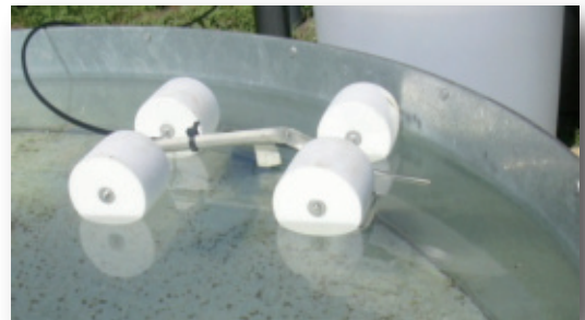
TS 265 sensor with float for evaporation tank
