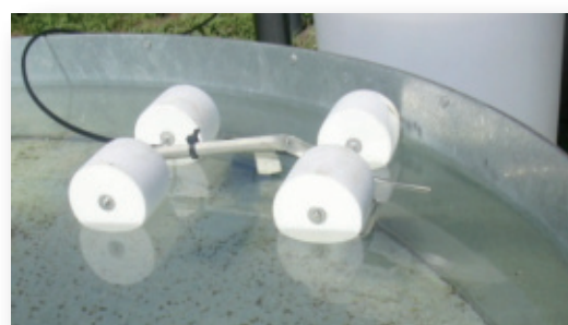
TS 265 sensor with float for evaporation tank
