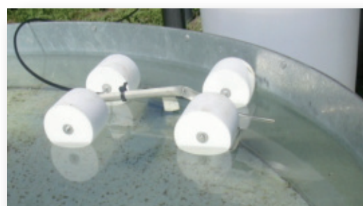
TS 265 sensor with float for evaporation tank
