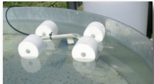
TS 265 sensor with float for evaporation tank
