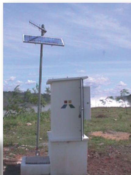
Measuring station of the Hydrometeorological Monitoring Network of ITaipu, Brazil-Paraguay
