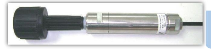
The TECMES sensor, Model TS 330, is a submersible type sensor for the measurement of dissolved oxygen in rivers, reservoirs, treatment plants, etc.
