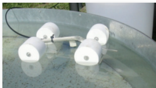
TS 265 sensor with float for evaporation tank
